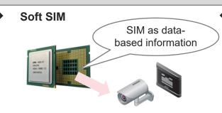
A communication module given SIM functions where the information required for mobile communications is logically written in internal memory eSIM (embedded SIM)
